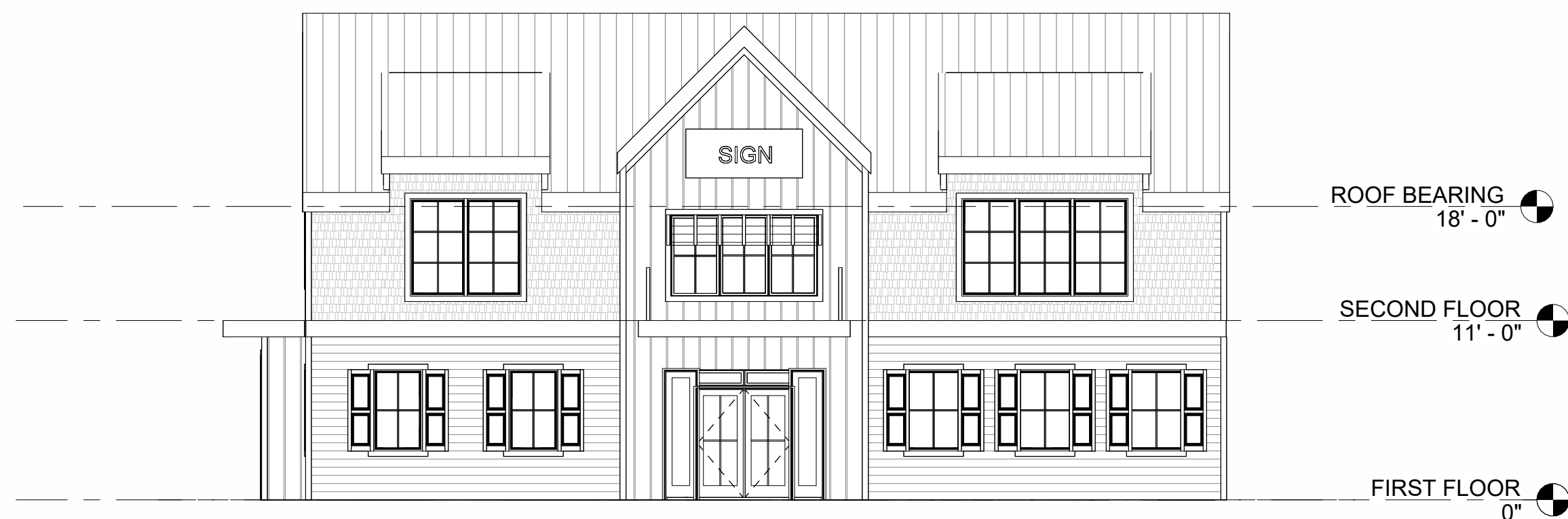
④ PROPOSED ELEVATION - ATLANTIC AVENUE 1/8" = 1'-0"
